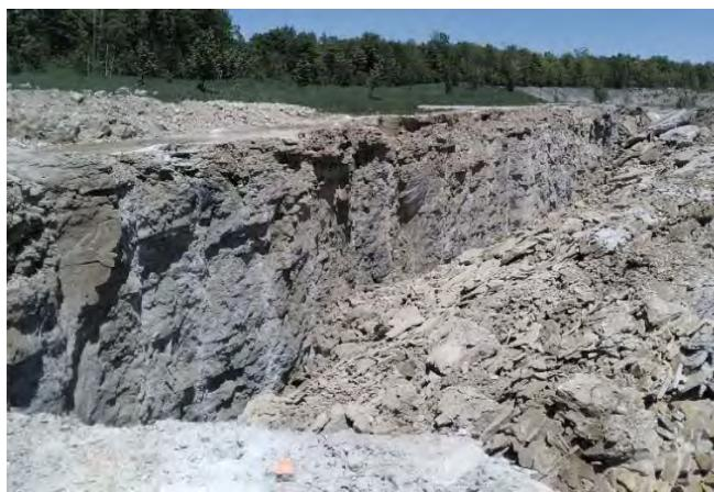
The AMP requires visual inspections along the active quarry face after each blast for water-bearing fractures. The intent is to ensure that the quarry does not interfere with potential epi-karst pathways that might otherwise deliver water to surface water features such as springs found in the Shouldice Wetland. Visual inspections were made by HSCL staff after each blast in 2018.
